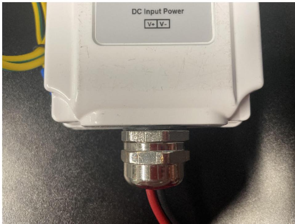
**Installation note:** Always connect the PoE case ground terminal wire to a Chassis or Earth ground during installation to protect the device.
